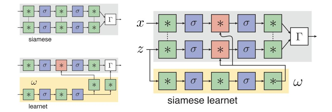
$$f(z,x) = \Gamma(\varphi(x; \omega(z; W')), \varphi(z; \omega(z; W')))$$
